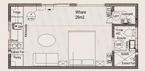
Materials include timber frame, ply floor and interior linings, color steel cladding to sides and rear (for durability, cost and low maintenance) and a timber/board and batten front wall.
