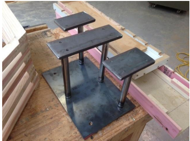
Figure 10. Mock-up #3 - connector plates
