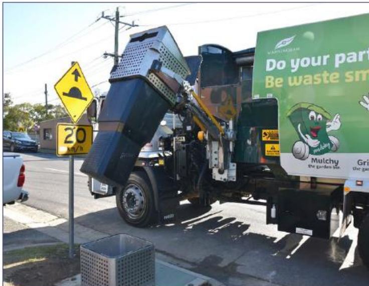
Figure 5-9 Automated emptying of a Riversafe bin. Source: 2018 ZAM-WSUD Handbook.
