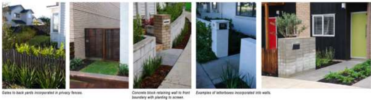
Figure 10. Design Guide principles example from the Sunderland Comprehensive Development Plan, for street-dwelling interfaces, gates, walls and letterboxes. 44
